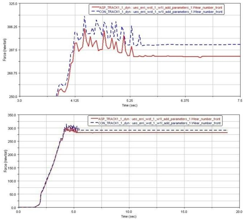
**Figure (6) Wear number-wagon with air spring (continuous line) and conventional wagon (dash line)**
