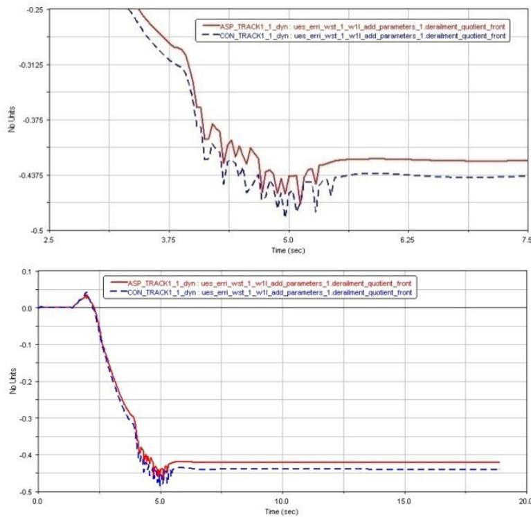
**Figure (9) Derailment index-wagon with air spring (continuous line) and conventional wagon (dash line)**
