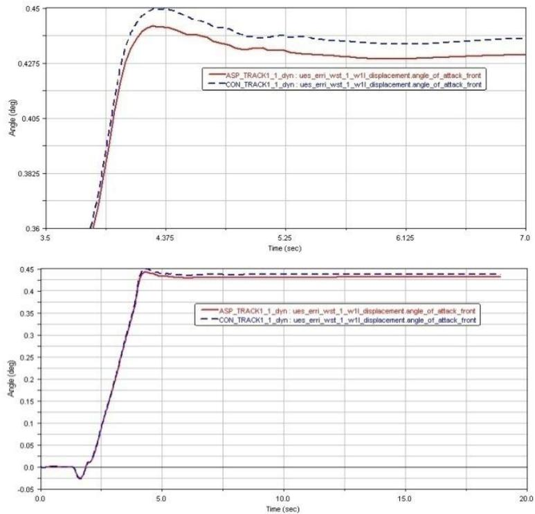
**Figure (7) Displacement angle-wagon with air spring (continuous line) and conventional wagon (dash line)**
