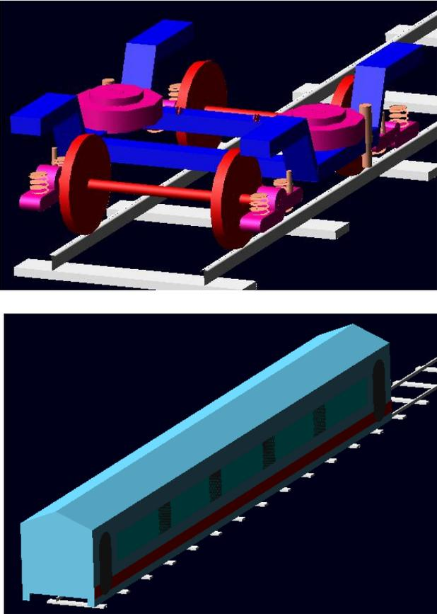
Figure (5) bogie and air spring that is modeled in Adams/Rail [1]
