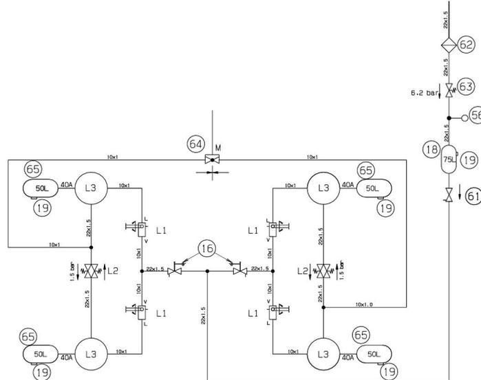
Figure (3) Air spring pneumatic diagram of IRICO Rail Bus [3]
