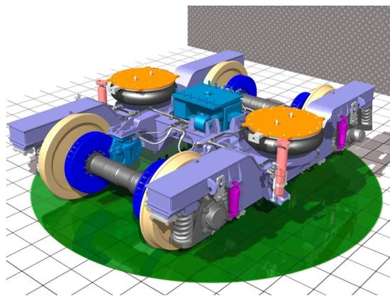
Figure (1) Bogie-IRICO Rail Bus [5]
