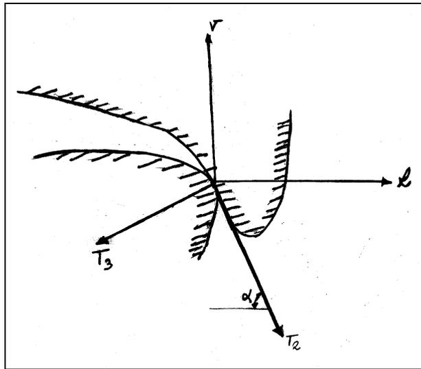
Figure (8) Contact forces that is used in NADAL theory
